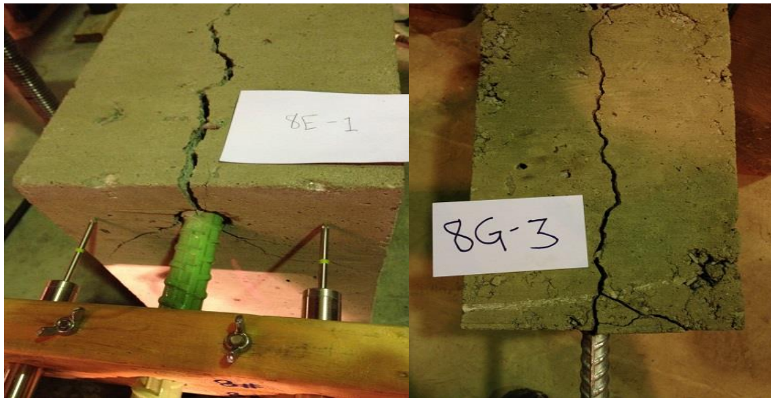
(a) Specimen with #8 epoxy coated test bar
